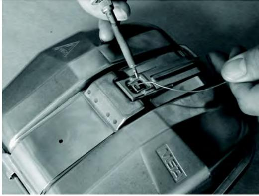
**Fig. 31** Affix lead seal (lead seal according to spare parts list).
