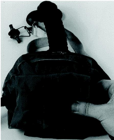
**Fig. 22** Fold lower side of the breathing bag twice from the bottom to the top (valve underneath canister bottom)
