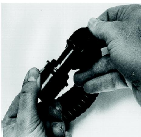
**Fig. 16** Insert connecting piece into the lowest fold of the breathing tube
