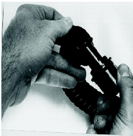
**Fig. 11** Remove connecting piece from breathing tube.
