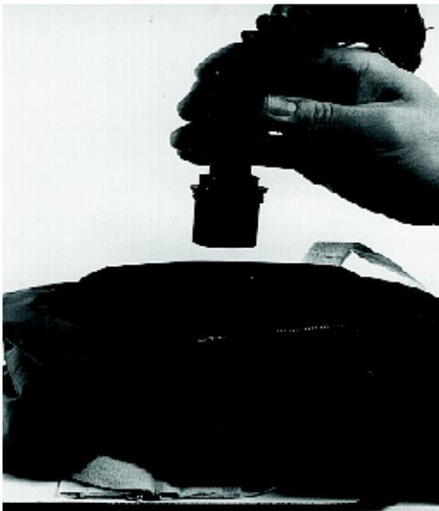
**Fig. 18** Screw breathing tube with connecting piece onto the canister. Adjust mouth-piece to body side.
