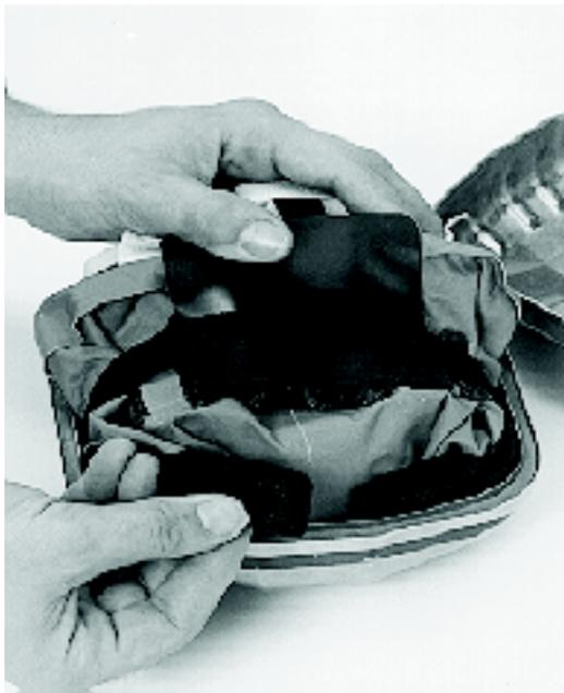
**Fig. 28** Fold together shorter end of waist belt and place it into case next to the valve. Repeat with remaining part of long end of waist belt.
