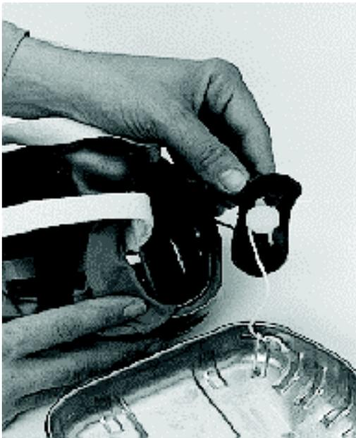
**Fig. 26** Insert mouthpiece plug into mouthpiece. Place mouthpiece into free space next to nose clip at case edge.
