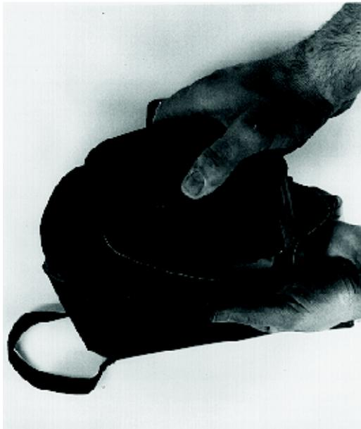
**Fig. 13** Pull out protective cover with canister from breathing bag.
