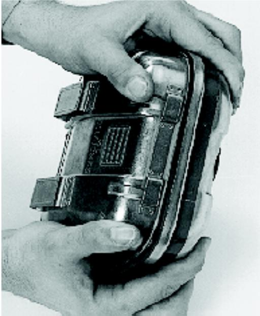
**Fig. 29** Place lower case onto unit. The belt loops are opposite the pressure compensation opening.
