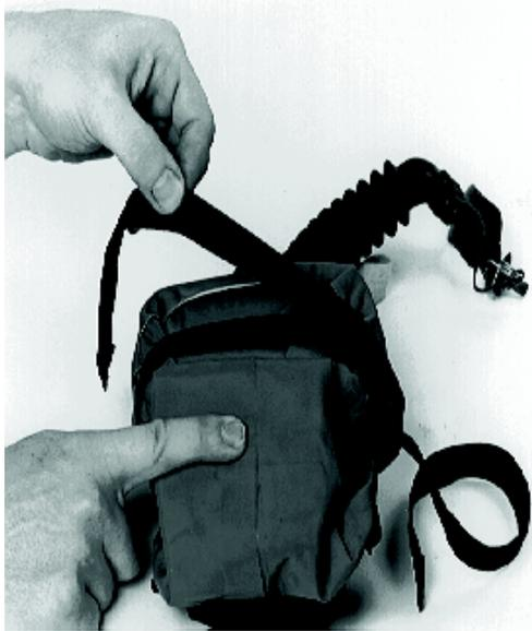
**Fig. 23** Hold folded breathing bag and wrap long end of waist belt once around the unit and pull tight
